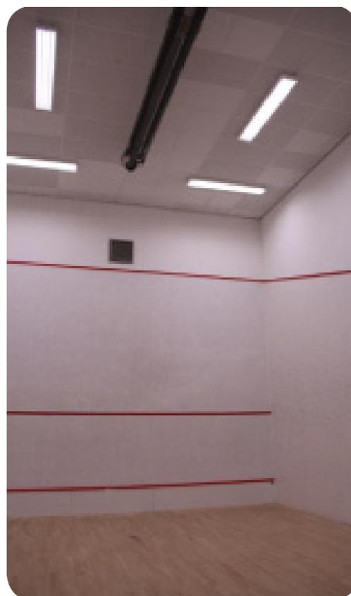
Squash court lit using LEDs controlled by PIR sensors
